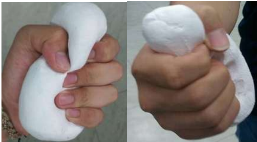
Figure 1. The acquirement of the complementary 3D surface of hand
